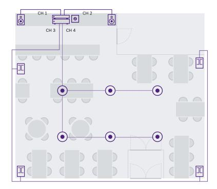
The layouts are for general and visual purposes only and should not be directly applied to any installation
