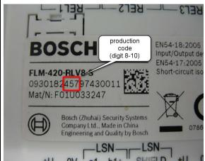
Additional to the functional test after manufacturing the PCBA, a complete functional test is currently performed at our distribution centre in Tilburg. This ensures that all FLM-420-RLV8-S modules currently leaving our distribution centre are 100% functional.
