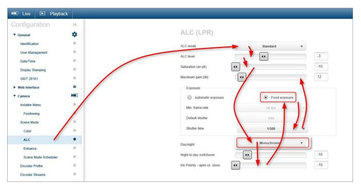
In ALC (LPR) capture scene mode at these shutter speeds, the camera will capture license plate images with sufficient contrast for ANPR (see figure 7).
