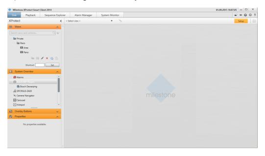
5. Drag and drop the **Bosch Dewarping** plug-in into an empty view item. The name of the plug-in will be shown in the upper left corner of the view.
