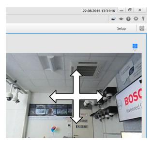
2. Hold the *right* mouse button and move the mouse up and down to control the zoom.
