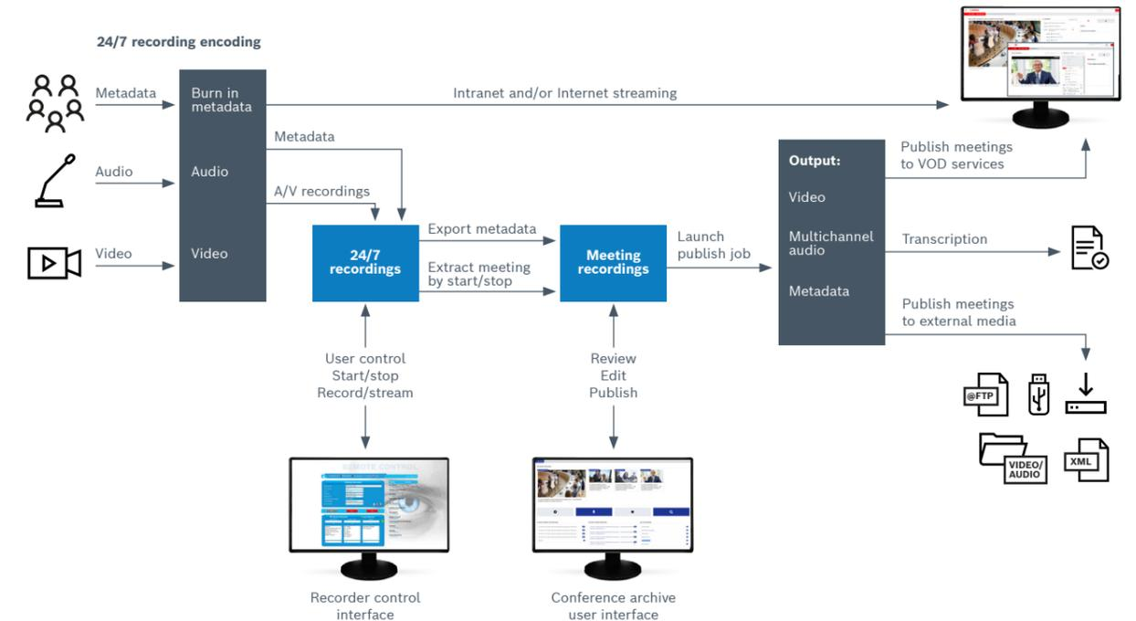
The IP-based DICENTIS Conference System from Bosch and the Arbor recording and archiving software are digitally interfaced by using the TCP-IP API protocol and DANTE™ audio technology.
