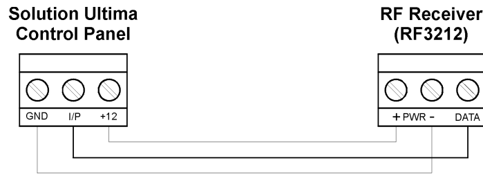
Figure 1: RF Receiver (RF3212) Wiring Diagram
