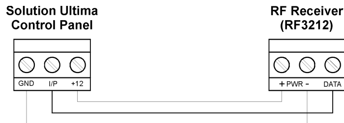
Figure 1: RF Receiver (RF3212) Wiring Diagram
