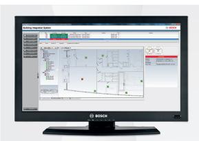
An alarm coming from a camera connected to XProtect can trigger alarm messages and automatic actions on the BIS server. All alarms are thus presented on one common alarm management dashboard.
