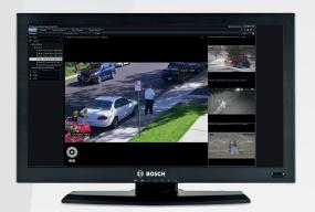
An alarm coming from a device or detector connected to the BIS server can trigger video verification of the alarm on XProtect client. The operator can then zoom in for details and further investigate the scene with more cameras before responding to the alarm.
