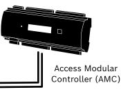
The base unit and controller share a Wiegand connection
