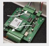
Step 1 Connect base unit to power, ground, Wiegand Data 0, Wiegand Data 1, LED, and Relay 1 input; then to Bosch AMC
