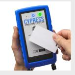
**Step 4** Test configuration by swiping credential on handheld unit. Green LED will be lit for access granted; red LED for access denied
