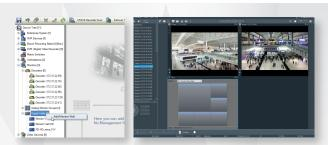
Create a 'Digital Wall' in BVMS and assign the RCP+-Decoder to it.
