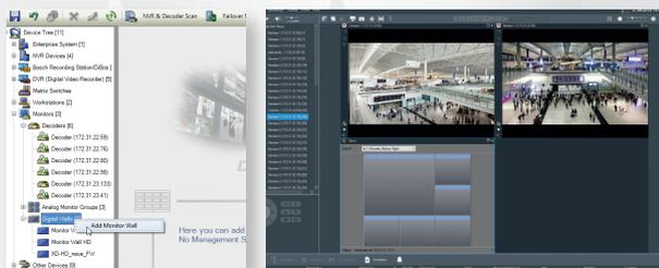
Create a 'Digital Wall' in BVMS and assign the RCP+-Decoder to it. A CMS 'Perspective' will automatically be created for this 'Digital Wall'
