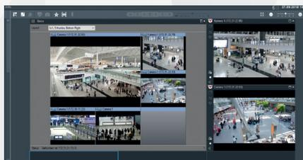
In BVMS Operator Client the operator has symbols for cameras and monitors (or a digital monitor wall) that represent the real cameras and monitors. When dragging a camera symbol onto a monitor symbol the BVMS system makes sure that the image of the real camera is displayed on the video wall.
