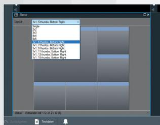
Different pre-defined layouts can be applied by the operator to the 'Digital Wall' to arrange various 'sources'. An operator can then drag 'Cameras' to 'Digital Wall' in the Operator Client, which then would be available as 'Sources' in CMS, and automatically placed in the CMS 'Perspective'.
