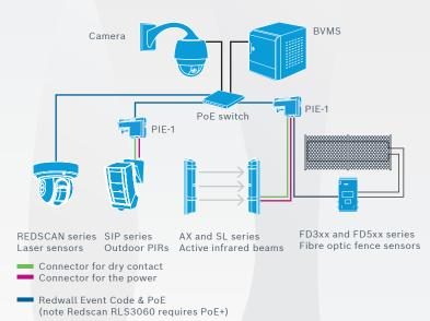
BVMS meets Optex IP motion and object detectors to provide reliable event triggered security systems to protect perimeters, approach, buildings, roofs and valuable or critical assets.
