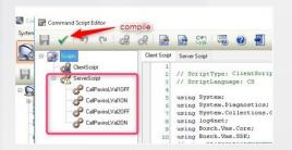
The Bosch Video Management Script editor is used to create a script which connects to the Bosch PAVIRO Public Address and Voice Alarm System. The script will link BVMS events to dedicated PAVIRO calls or messages and sends these to PAVIRO's target zones. The script will be supplied by Bosch Security and Safety Systems on request.
