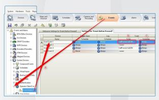
The BVMS alarm management configuration allows to trigger an announcement by selecting a specific script as an action on an incoming event. This can be a Video Content Analysis event, as well as an event triggered by a third party system (for example fence detection).
