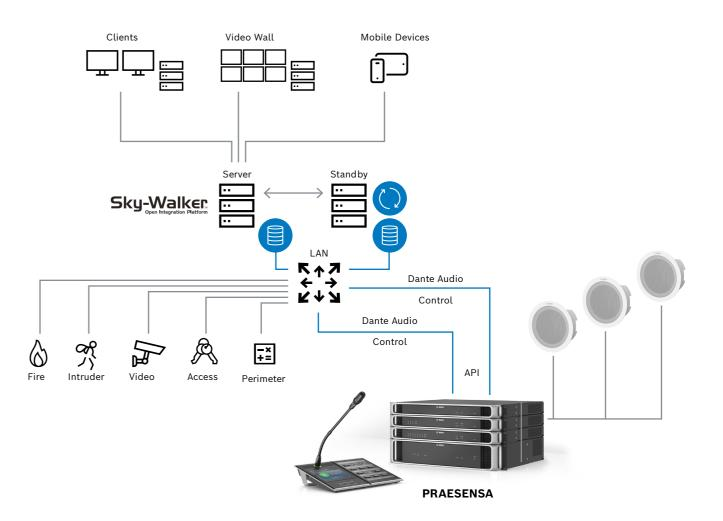
The PRAESENSA Public Address and Voice Alarm system by Bosch and the Sky-Walker PSIM software platform by Entelec are linked via AES67/Dante audio streaming and TCP/IP control.
